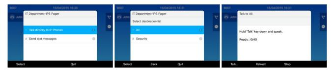
Audio is played on Cisco IP Phones's speakers. If the IP phone is engaged on a call, the internal calling party will hear the audio message from the handset. It is also possible to play audio message on IP Speakers, like CyberData or Algo Solution SIP-enabled IP Speaker.
