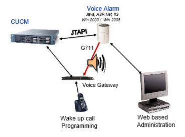
To program a wake up call, the user rings a directory number (may be a short number). The application detects the calling number, which will be used to call back. It should be noted that if the calling number is a shared line, the phones sharing the line will be both called back by Voice Alarm.
